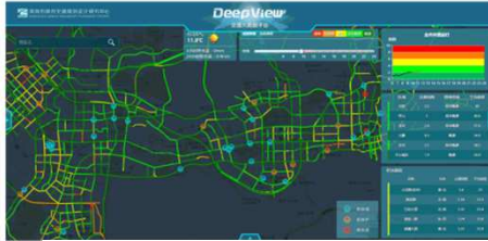
Road traffic operating index system
